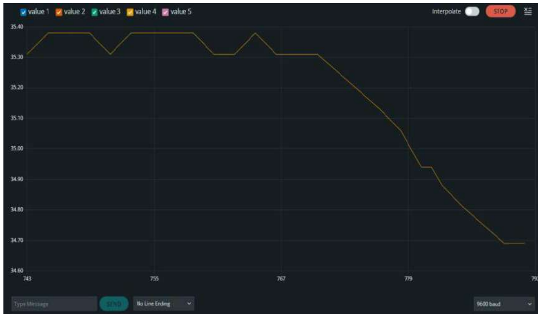
Figure(3.19) Thermal profile showing decrease in temperature when the probe is placed away from the heat source.
