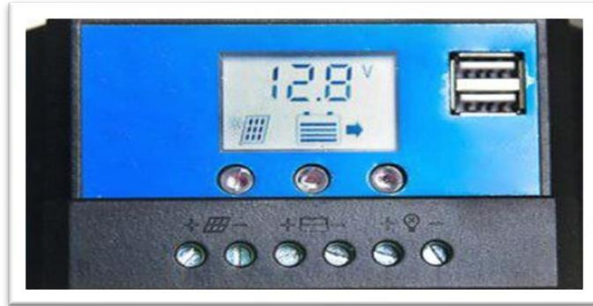
Figure 3.5: Solar power controller
